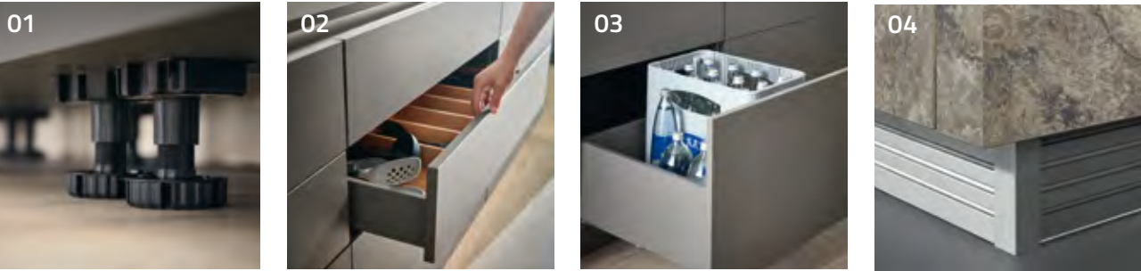
01. The positioning of the plinth feet can be adjusted if required. Height adjustment +18/-10 mm. 02. – 03. Further advantages of the 133 mm grid is that, for example, both a soup ladle and a water crate can easily be accommodated. 04. Lamella base – ventilation for built-in devices, for example hob extractors.
